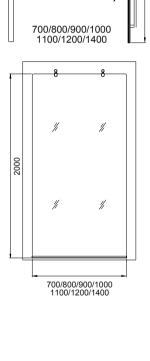
All measurements shown are in millimetres. Drawing sizes are not to scale. Measurement accuracy  $\pm 5 \text{mm}.$
